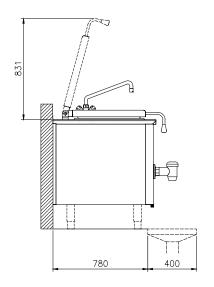
Cold Water inlet 1 (cleaning) ΕI Electrical inlet (power) HWI Hot water inlet
